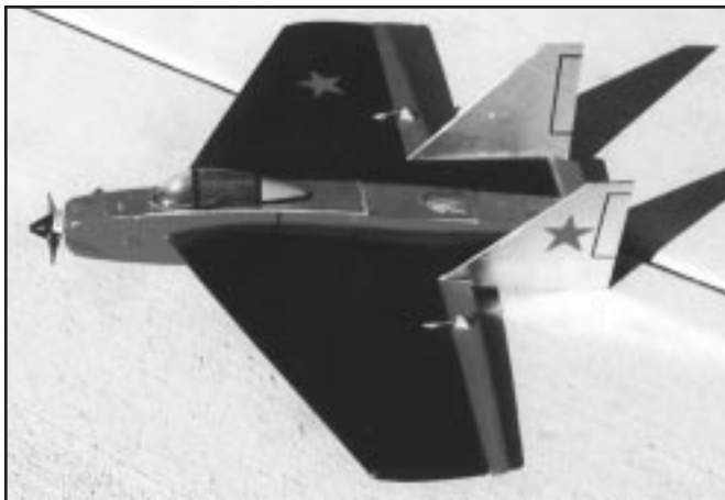
Adam Kremers' newest plane, a Lanier Shrike. It flies better with a direct drive sp400 than with a ducted fan. 16 oz. rtf on 8 cells.
