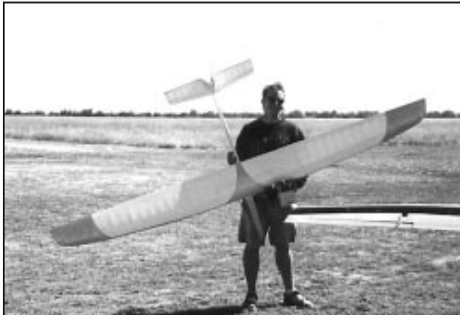
Ron Marston with his freshly rebuilt 120" RES ship. 75 oz. and about 1200 sq. in.
