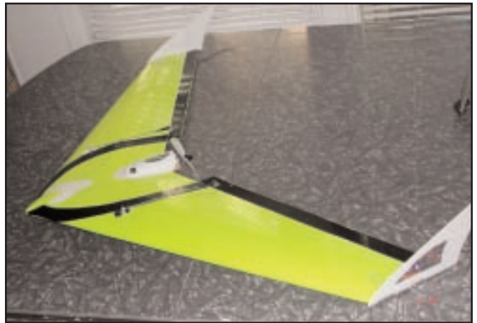
Ron's new Wedgie. Thinner and lighter (15.5 oz.) than a Zagi or Razor.
