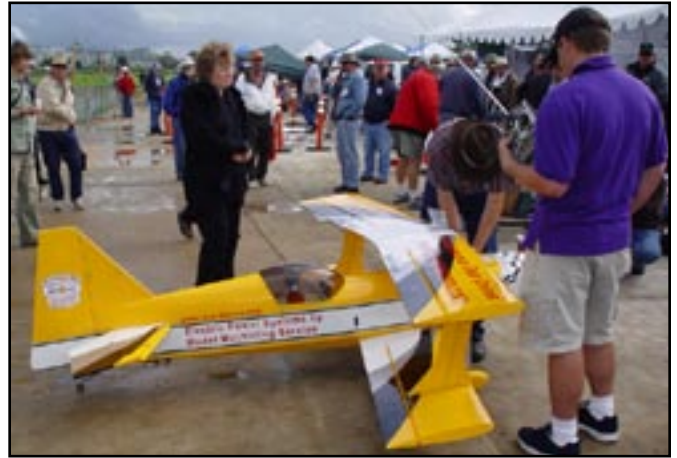
46% Ultimate Bipe. with a 32" prop powered by 4 large Hacker motors on an inner driven gearbox and a really expensive wad of Thunder Power LiPoly batteries. This plane hovered on the prop at about 2/3 throttle.
