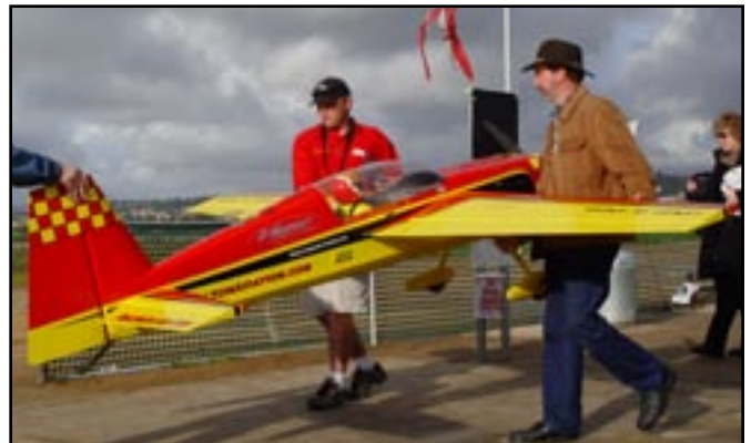
43% Extra 300 (I think) with a 28" prop and 4 large Hacker motors. Very impressive performance. Pilot for this plane and the Bipe above is 23 year old Mark Leseberg Jr., who is also an accomplished full scale pilot.
